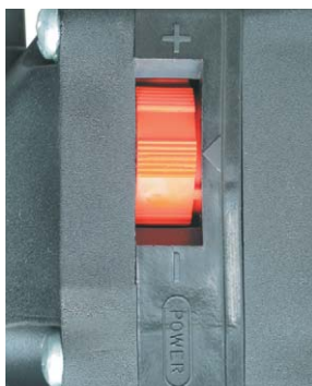
Drehmomentvoreinstellung Torque pre-selection: EHB 32/2.2 R R/L
